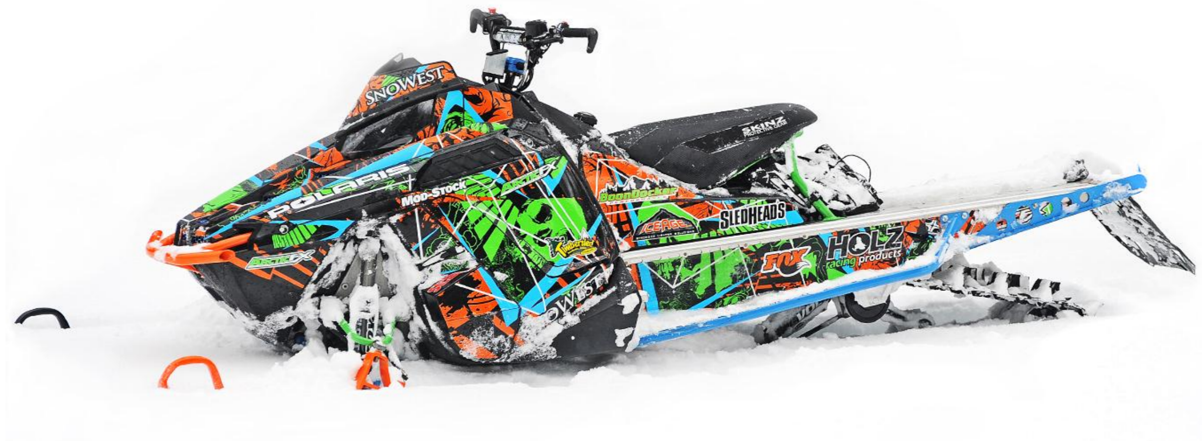
Graphics printed with the GERBER EDGE® on Convex® High-Bond™ 6 mil white with Convex® 8 mil conformable laminate.
