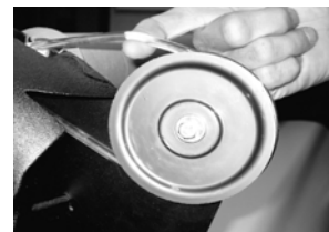
4. install belt on pulleys
