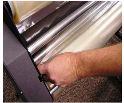
Tacking laminate from top roll to exposed adhesive on bottom roll
