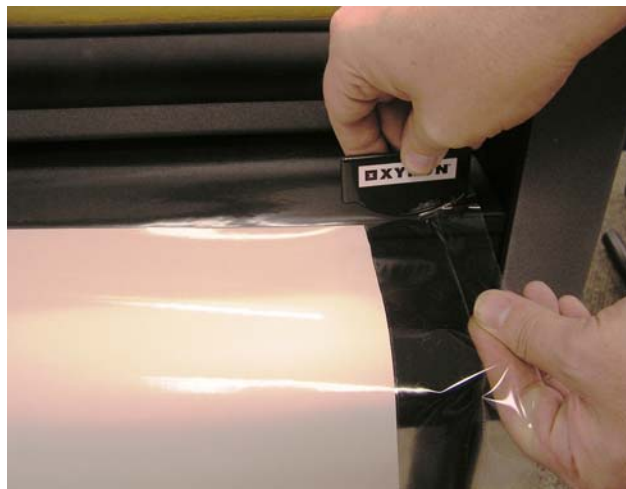
Apply tension to film when cutting
