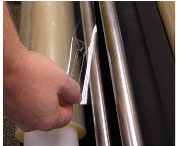
Insert the Top and Bottom roll as shown
