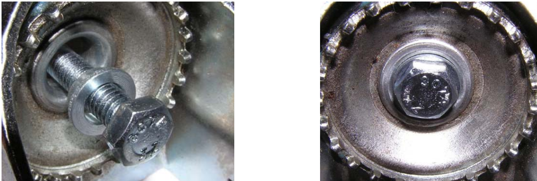
Figure 4/5: Using hardware supplied, secure caster frame to cart
